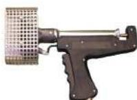
**Heat Gun** Powered by propane gas, the heat gun is designed to give a tight, consistent finish to the shrink wrap covering. This tool is very reliable and is supplied with a regulator and 8m hose. We also supply the Ripack 2200 heat gun which has a range of extensions available to allow an operator to safely reach up to 2m. A heat gun extension is essential for shrinkwrapping larger products.
