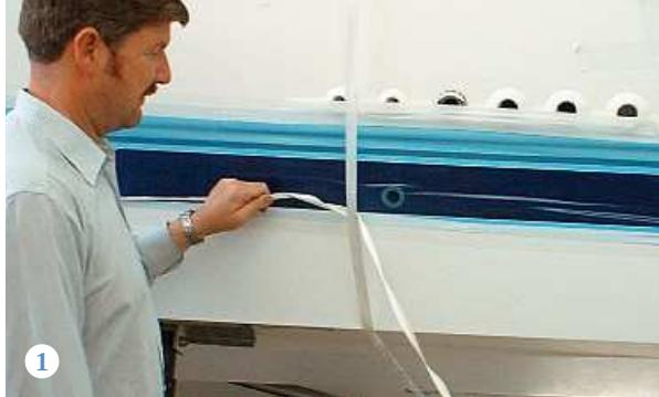
**Step 2** – The roll of shrink wrap is placed on a stand so that it can be easily unrolled. The shrink wrap is then pulled over the product, cut from the roll and unfolded.
