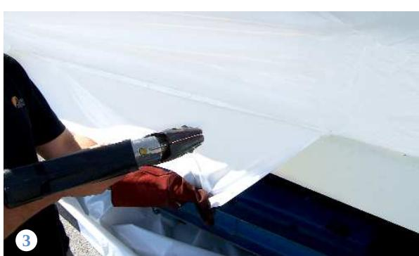
**Step 4** – Once the perimeter band has been 'welded' and any pleats sealed, the entire cover may be shrunk. Begin at the bottom and shrink upward using strokes similar to spray-painting.
