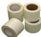
**Patch Tape Rolls** 100mm wide, high tack adhesive, waterproof. Used for repairing small holes and holding seams and large patches in position. For smaller boats, tape can also be used for securing the shrink wrap to the hull of the boat rather than using a perimeter band.
