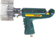
**Heat Gun** Powered by propane gas, the heat gun is designed to give a tight, consistent finish to the shrink wrap covering. This tool is very reliable and is supplied with a regulator and 8m hose. We also supply the Ripack 2200 heat gun which has a range of extensions available to allow an operator to safely reach up to 2m. A heat gun extension is essential for shrinkwrapping larger fly-bridge type boats.
