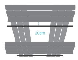
**Roof sheeting rails** must be installed beneath the perpendicular boards 20cm away from boards to secure sheets.
