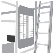
**Roof access** should be via ladder and safety access gate, at the side of the roof. Where access is provided through the roof there is a risk of leaks in the completed job.
