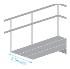
A **run of 3 boards** should be installed around the perimeter of the roof, please leave the toe board off to ensure that the sheeting runs smoothly over the edge.
